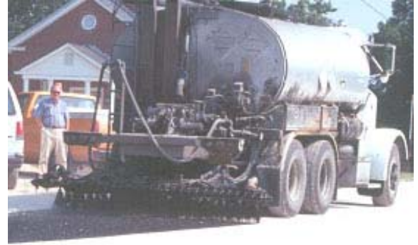
Figure 2 – Asphalt Distributor Truck
